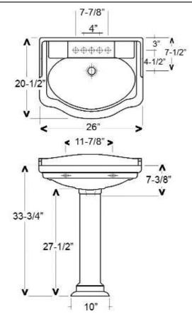
Dimensions of fixture are nominal and may vary within the range of tolerances established by ASME Standard A112.19.2-2018. Dimensions and specifications subject to change without notice.
